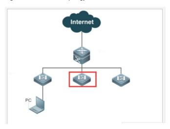
Note: The device enclosed in the red frame in the preceding figure is the accessed switch. If the switch can be pinged successfully from the PC, you can access the eWeb management system deployed on the switch.
